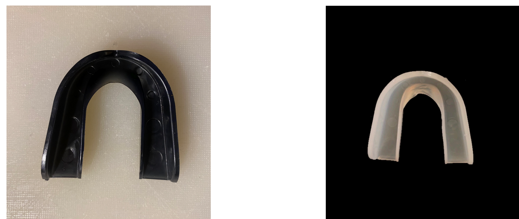
Figure 2. On the left is a photo of the mouth guard at room temperature. On the right is a photo of the mouth guard after being heated in boiling water to 39°C.
